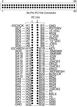
Figure PC104: 64-Pin PC/104 Connector Bus A & B
